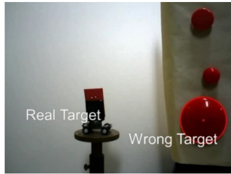
Figure 5. 17 Camera recognized other object with the same color in visible spectrum.
