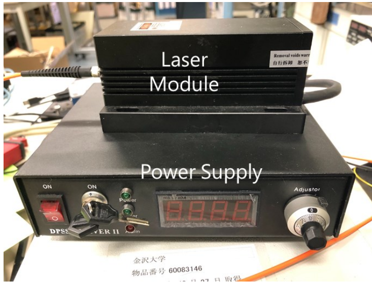
Figure 5. 4 Picture of laser module and power supply.
