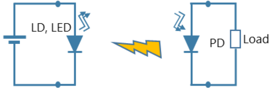
Figure 3. 1 Basic diagram of OWPT system.
