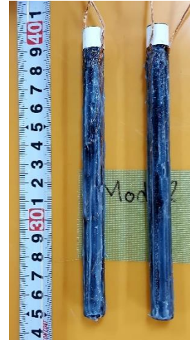
(b) model piles after covering silicone
