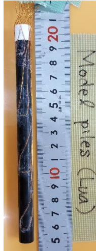
(a) a model pile after attaching strain gages
