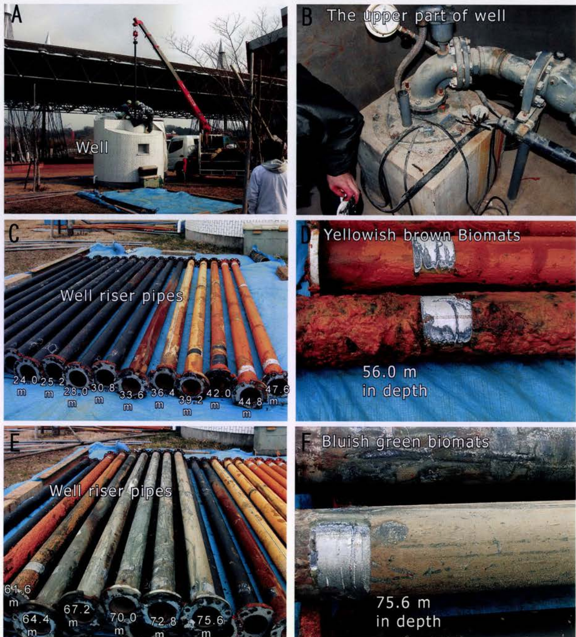
Fig.2 Photographs of sampling location during dredging operations and microbial mats on outer surfaces of well riser pipes on March 8th, 2005. A: Pulling up of well riser pipes. B: The upper part of well in an establishment. C: Yellowish brown microbial mats form on the parts deeper than 30.8 m. D: Thick yellowish brown microbial mats in 56.0 m depth (Thickness: 5 mm). E: Bluish green microbial mats form on the parts deeper than 61.6 m. F: Bluish green microbial mats in 75.6 m depth.
