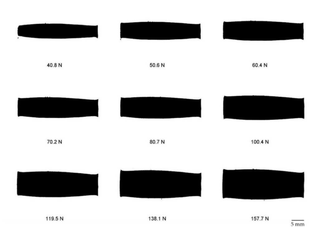
Figure 4.12 Fluorescence images of rubber-wheel apparent contact due to applied normal loads (images belong to trial 2)
