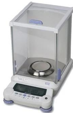
Fig. 3-35. Analytical balance for measuring mass [104].
