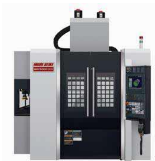
Fig. 3-17. Appearance of the 5-axis machining center NMV5000 DCG [90].
