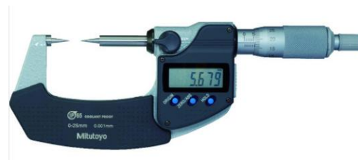
Fig. 3-36. Micrometer for measuring length [105].
