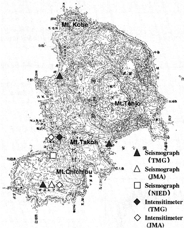
Fig.2 Locations of seismographs and seismic intensity instruments
