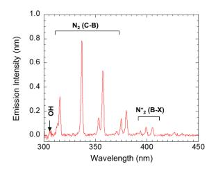
Figure 4. OES of RE-DBDR at  $f_{app}$  = 60 Hz,  $V_{pp}$  = 30 kV, and 5000 rpm rotational speed.
