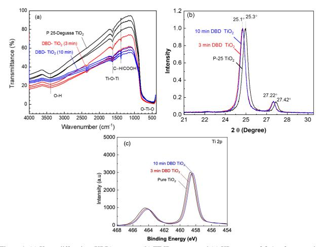
Figure 4: (a) X-ray diffraction (XRD) patterns, (b) FT-IR spectra, and (c) XP spectra of O 1s of untreated TiO<sub>2</sub> and when TiO<sub>2</sub> nano-powder was treated for 3 min and 10 min at  $f_{app}$ = 60 Hz,  $V_{pp}$ = 30 kV, and rotational speed = 5000 rpm
