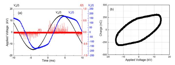
Figure 2. Electrical characteristic of RE-DBDR. (a) Voltage and current waveforms of (RE-DBDR), I(t) is discharge current,  $V_a(t)$  is applied voltage, and  $V_c(t)$  is capacitance voltage; (b) Lissajous figure at  $f_{app} = 60$  Hz,  $V_{pp} = 30$  kV, rotational speed = 5000 rpm.
