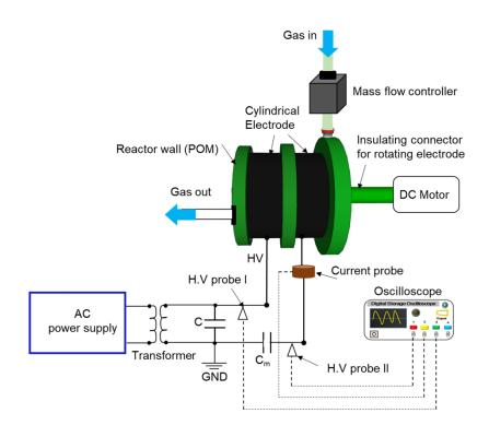
Figure 1. Experiment setup for rotary electrode dielectric barrier discharge reactor (RE-DBDR) An air compressor introduced air into the reactor. Gas flow rate was controlled using a mass flow controller
