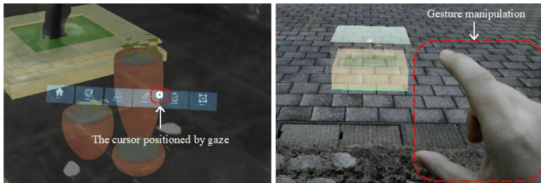
Fig. 2.3. Real-time manipulation of 3D models through HoloDesigner.
