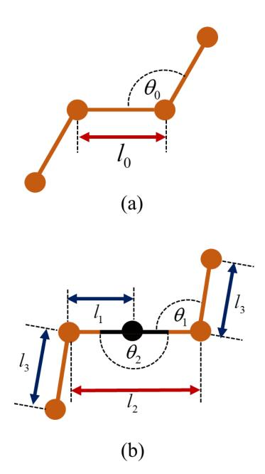
Fig. 1. (Color online) Geometries of pristine silicon (a) and muonium impurity at the BC site (b).  $\theta_0 = 109.5^0$  and  $l_0=2.35$  Å respectively. The silicon and muonium atoms are denoted by the light brown sphere and dark sphere, respectively.
