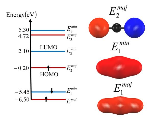
**Fig. 7.** (Color online) Schematic diagram of energies of the linear tri-hydrogen molecule on the lefthand side and wavefunctions on the righthand side where the red and blue colors represent positive and negative amplitudes, respectively.
