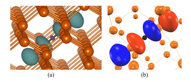
**Fig. 4.** (Color online) (a) Spin density where the absolute value of the isosurfaces is  $1.50 \times 10^{-3}$  bohr<sup>-3</sup>. The positive and negative spin densities are represented by green and purple colors, respectively. (b) Wavefunction of the impurity level. The red and blue colors represent positive and negative values, respectively.
