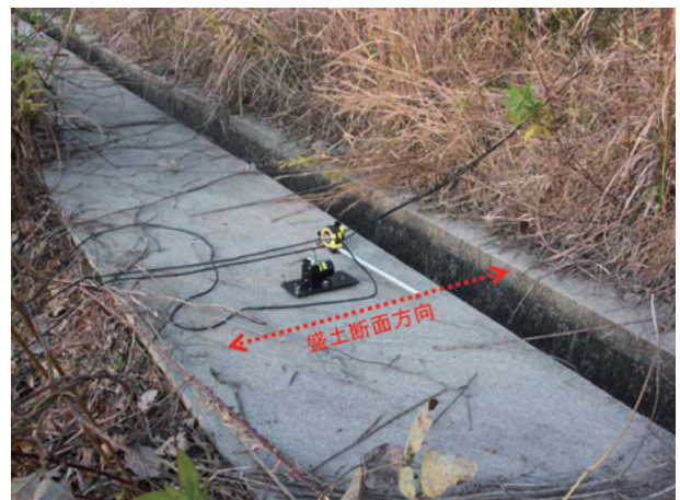
写真-3 常時微動計測状況 (P-5地点) Photo 3 A microtremor measurement condition. (P-5 site)
