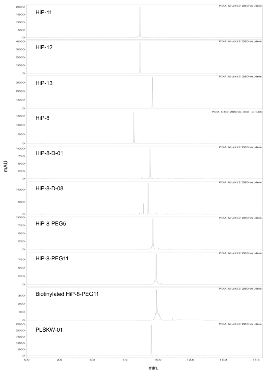
Supplementary Figure 21 | Analytical UHPLC of chemically synthesized peptides. Approximately 1 nmol of peptide was analyzed by UHPLC on a 10-70 vol% aqueous acetonitrile gradient, with intensity monitored by absorbance at 280 nm. These experiments were repeated twice independently with similar results.
