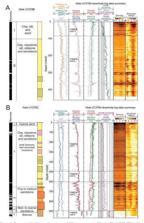
Figure 5. Summary of the lithostratigraphy and LWD measurements. [A] is for Site U1378, [B] for Site 1379C. GVR=geoVISION tool, ARC=arcVISION tool, PEF=photoelectric factor, IDRO=image-derived density (EcoScope tool), RHOB=bulk density, RING=resistivity measured by the ring electrode (geoVISION tool), P16B=phase-shift resistivity measured at a 16-inch source-receiver separation (arcVISION tool), A40B=attenuation resistivity measured at a 40-inch source-receiver separation (arcVISION tool).
