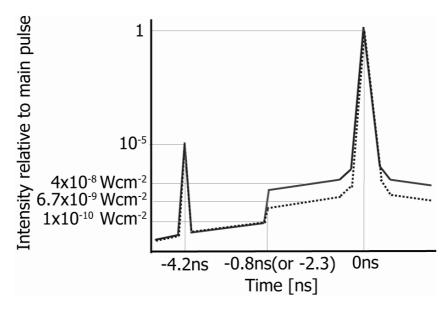
**FIGURE 7.** Condition of the pre-pulse which is the leakage from the regenerative amplifier and ASE pedestals. The ASE pedestals change their intensity at the time of the switching time of the Pockels cell (-0.8ns). The measured condition is shown with the solid line (hereafter condition-1), which is the case for the copper target. The effective condition (hereafter condition-2) is shown with the dotted-line, which is the case for the Polyimide targets.
