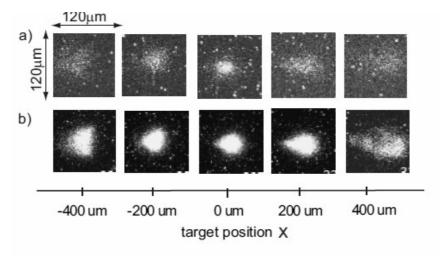
FIGURE 2. Soft x-ray (≥1 keV) images of the target front surface of a) Polyimide 7.5 μm and b) copper 5 μm targets, depending on the target position. Position 0.0 μm corresponds to the position where the proton spectra shows maximum energies of ~4 MeV. At position 0.0 μm, the plasma size seen in the x-ray images takes the minimum size. We observed brighter and smaller in size x-ray spots for the case of copper target than that of the Polyimide target.
