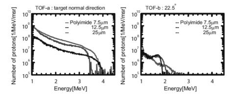
FIGURE 3. Typical energy spectra of protons observed by the time-of-flight (TOF) spectrometer. Panel a) shows the data from TOF-0° installed at target normal direction and panel b) from TOF-22.5° at 22.5° from the target normal direction. In both panels, red, black, and blue lines show the data with  $7.5\mu m, \, 12.5\mu m, \, and \, 25\mu m$ -target, respectively.
