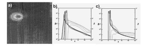
**FIGURE 8.** (a)Typical plasma image from interferometer with the 800-nm probe 50ps before the mainpulse arrival for the 7.5μm-Polyimide target. (b)The electron density profiles at initial time (rectangular profile) and just before the main pulse arrival with the ASE condition-1. (c) Same as (b) but with ASE condition-2.
