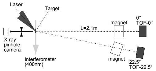
**FIGURE 1.** Experimental setup. "TOF" stands for time of flight proton energy spectrometer. TOF-0° and TOF-22.5° represent one which is placed normal to the target rear surface and at 22.5° from the normal.
