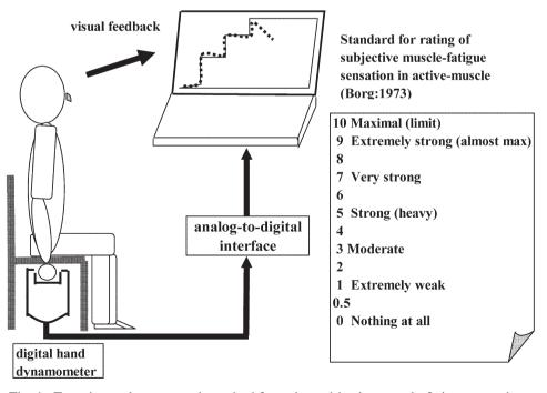
Fig. 1. Experimental system and standard for rating subjective muscle-fatigue sensation.
