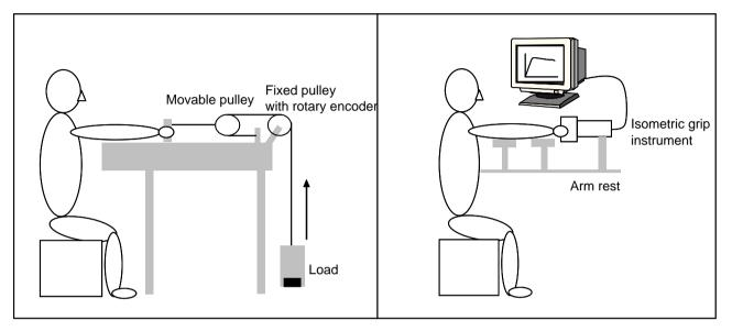
Fig. 1 Overview of the two grip tests (left panel: power grip, right panel: explosive isometric grip).
