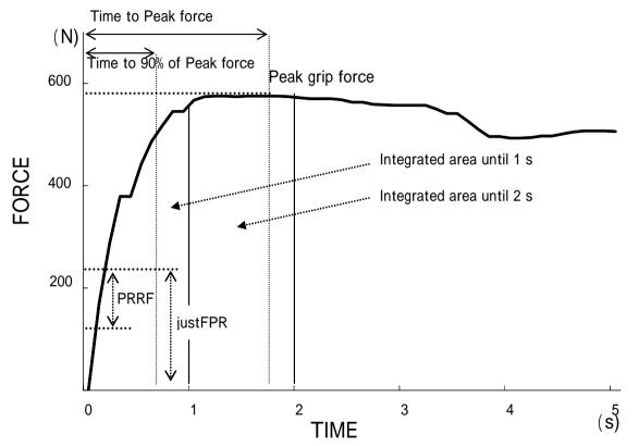
Fig. 3 Force-time parameters in the explosive isometric grip test. PRRF: peak rate of rising force, just FPR: force when peak rate of force appeared. The average forces to 90% and 100% of peak force were calculated by dividing the integrated area by time.
