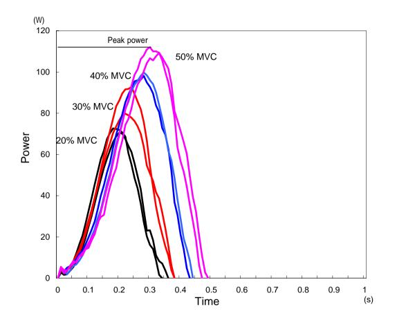
Fig. 2 Average curve of the power in the power grip test. Power = load (kg) × gravitational acceleration  $(9.80665 \text{m/s}^2)$  × velocity in each sampling (m/s)
