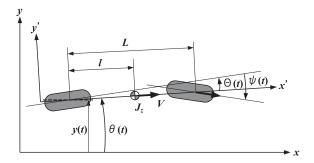
Fig. 3. The two-wheeled vehicle shifted from the course
