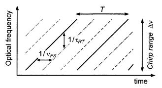
Fig. 3. Schematic drawing of the chirped frequency comb. Three modes are simultaneously frequency chirped in this drawing.
