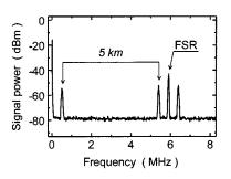
Fig. 7. Measured beat spectrum for a 5-km-long optical fiber.
