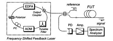
Fig. 2. System configuration for measuring the chromatic dispersion by means of optical ranging system using a FSF laser.
