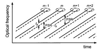
Fig. 6. Schematic drawing of the instantaneous optial frequencies of the reference beam (solid line) and the signal beam (dashed line) with the mode number labeled with (m - 1)-(m + 2).
