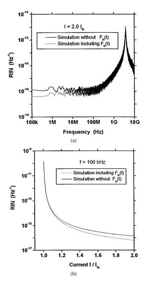
Fig. 9. Effect of ignoring the carrier noise source  $F_N(t)$  on the: (a) spectrum of RIN at  $I=2.0I_{th}$  and (b) RIN values at the low frequency of 100 kHz. RIN is overestimated when  $F_N(t)=0$  in the low-frequency regime at injection levels far from threshold.
