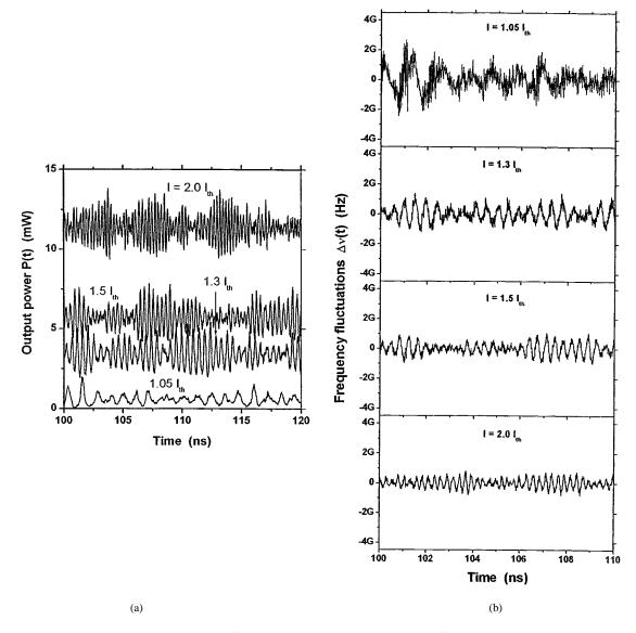
Fig. 5. Instantaneous fluctuations of: (a) the output power P(t) and (b) the oscillating frequency shift  $\Delta\nu(t)$  far from the relaxation regime at different injection currents. The fluctuations are suppressed while their repetition becomes faster when I increases.
