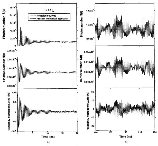
Fig. 3. Time-variations of the photon number S(t), the carrier number N(t), and the instantaneous frequency fluctuations  $\Delta \nu(t)$ : (a) during transients and (b) after termination of transients. Characteristics without the noise sources  $F_S(t)$ ,  $F_{\theta}(t)$ , and  $F_N(t)$  (dashed lines) are included for comparison. These quantities fluctuate around their dc values even after the termination of transients.
