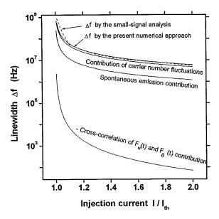
Fig. 8. Variation of the linewidth  $\Delta f$  with current I at a frequency as low as 100 kHz. The corresponding variations of the mechanisms contributing to broadening of  $\Delta f$  are also shown. The figure shows the rapid narrowing of  $\Delta f$  with increasing I near threshold.
