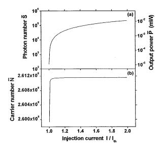
Fig. 2. Dependence of the dc values of: (a) the photon number  $\overline{S}$ , and (b) the carrier number  $\overline{N}$  on the injection current I. Corresponding L-I characteristics are also given in (a) with the right-hand vertical axis.
