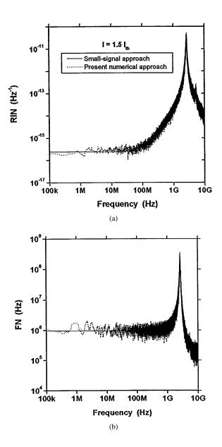
Fig. 4. Frequency spectra of: (a) quantum RIN and (b) quantum FN at injection current  $I=1.5I_{th}$ . The spectra peak around the resonance frequency  $f_r$  and are almost flat in the low-frequency regime. The characteristics are a good fit with those calculated by the small-signal analysis.
