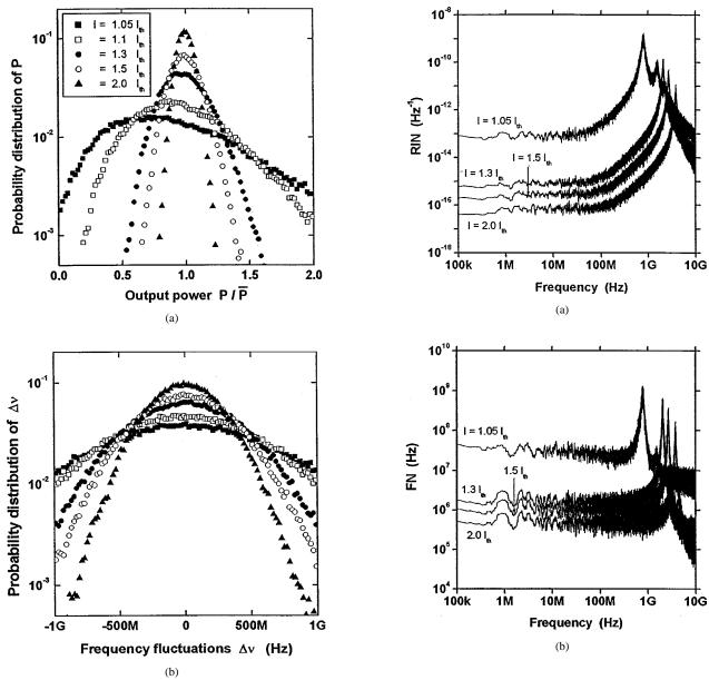
Fig. 6. The probability distributions of: (a) the output power P(t) and (b) the frequency fluctuations  $\Delta \nu(t)$  at different injection levels. High and narrow distributions are shown at high current values.
