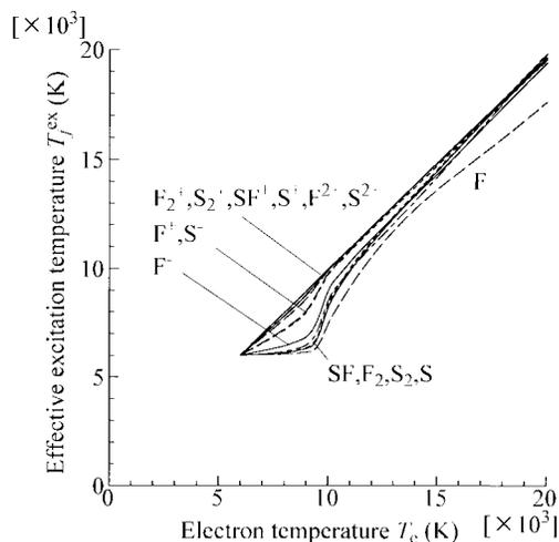
Fig. 4. Effective excitation temperature of various species in two-temperature SF<sub>6</sub> plasma at 0.1 MPa as a function of electron temperature. Gas temperature is fixed at 6000 K.
