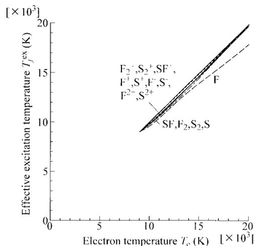
Fig. 6. Effective excitation temperature of various species in two-temperature SF<sub>6</sub> plasma at 0.1 MPa as a function of electron temperature. Gas temperature is fixed at 9000 K.
