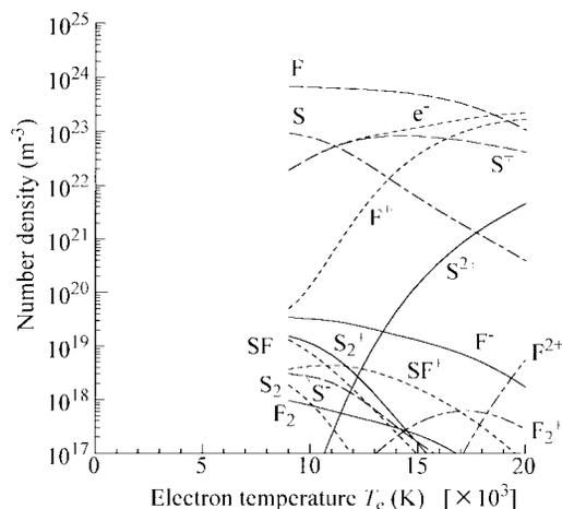
Fig. 5. Particle composition of two-temperature SF<sub>6</sub> plasma at 0.1 MPa as a function of electron temperature. Gas temperature is fixed at 9000 K.
