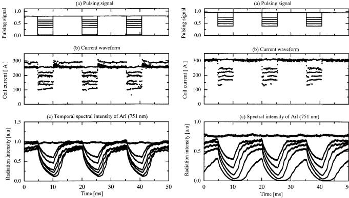
Fig. 9. (a) Spectroscopically measured temporal pulsing signal, (b) modulated current waveform peaks, and (c) radiation intensity of atomic argon at 10 mm below the coil-end for Ar plasma.
