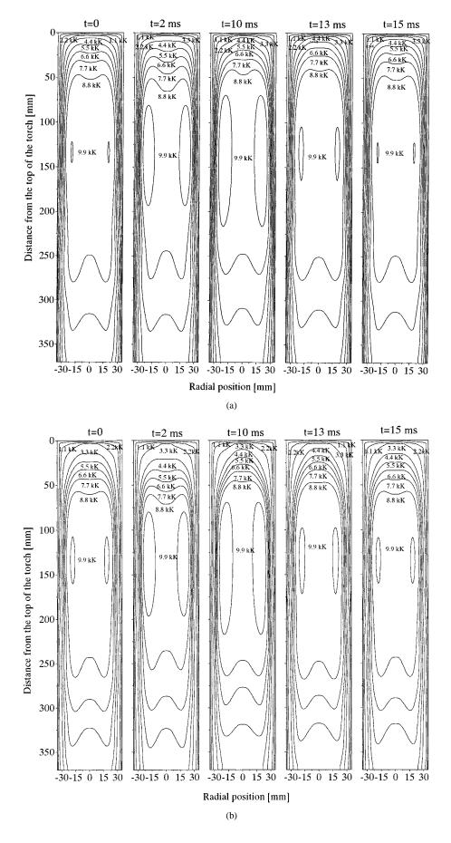
Fig. 3. Spatial distribution of temperature at 72% SCL for (a) Ar and (b) Ar-H<sub>2</sub> plasmas, at distinct time instants over a cycle of pulsing signal.
