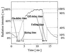
Fig. 8. Definitions of different response times of plasma.
