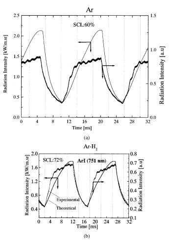
Fig. 12. Comparison of experimental and simulated radiation intensities of ArI (751 nm), for (a) Ar and (b) Ar– $\rm H_2$  plasmas, measured/predicted at 10 mm below the coil-end ( $z=2\,14$  mm).
