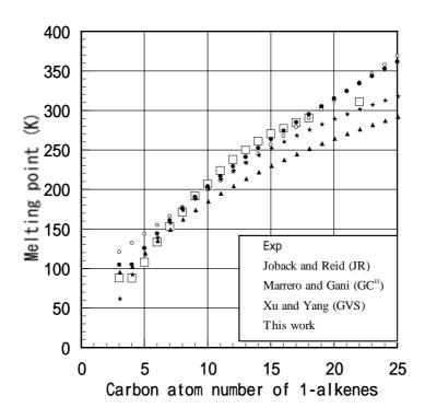
Fig. 7. Comparison of melting points of n-alkenes estimated by the present model with those obtained by previous models
