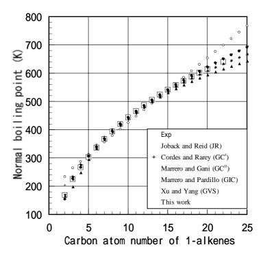
Fig. 3. Comparison of boiling points of 1-alkenes estimated by the present model with those obtained by previous models
