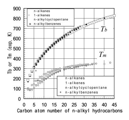
Fig. 10. Plots of experimental  $T_b$  and  $T_m$  against carbon number of n-alkyl hydrocarbons
