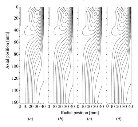
**Figure 12.** Streamline for Ar thermal plasma with injections of (a) PTFE, (b) PMMA, (c) PE, and (d) POM. The powder feed rate is 1 g min<sup>-1</sup>.
