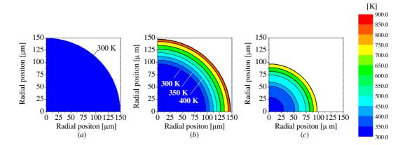
**Figure 6.** Time evolution in radial temperature distributions inside a test PTFE particle injected into Ar thermal plasmas: (a)  $t_{\rm p}{=}5$  ms,  $z_{\rm p}{=}9.20$  mm; (b)  $t_{\rm p}{=}25$  ms,  $z_{\rm p}{=}43.76$  mm; and (c)  $t_{\rm p}{=}30$  ms,  $z_{\rm p}{=}49.45$  mm, where  $t_{\rm p}$  is the time after particle injection, and  $z_{\rm p}$  is the axial position of a particle in the plasma torch.
