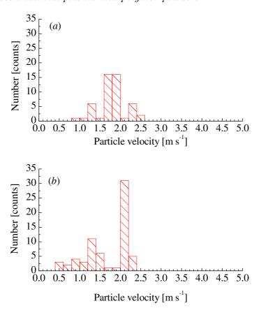
**Figure 16.** The experimentally measured and numerically calculated velocity distributions of injected PTFE particles into Ar thermal plasmas. The velocity distribution was estimated between the first and second coils of the plasma torch. (a) Experimentally measured (b) Numerically calculated
