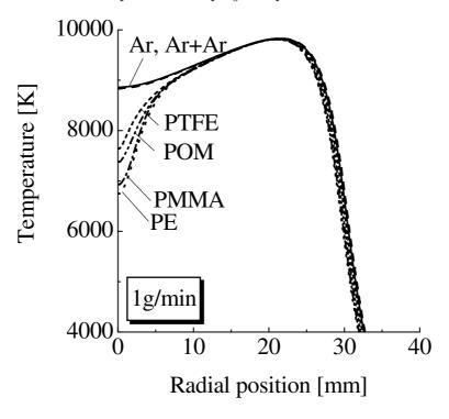
Figure 10. Radial temperature distributions of Ar thermal plasmas with polymer powder injections at the axial position of 95 mm. The powder feed rate is  $1 \text{ g min}^{-1}$ .
