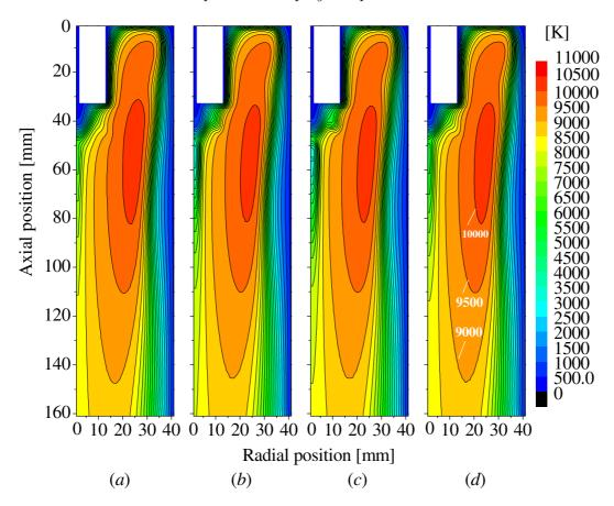
**Figure 9.** Temperature distributions of Ar thermal plasmas at atmospheric pressure with (a) PTFE, (b) PMMA, (c) PE, and (d) POM solid powder injections. The powder feed rate is  $1 \text{ g min}^{-1}$ .
