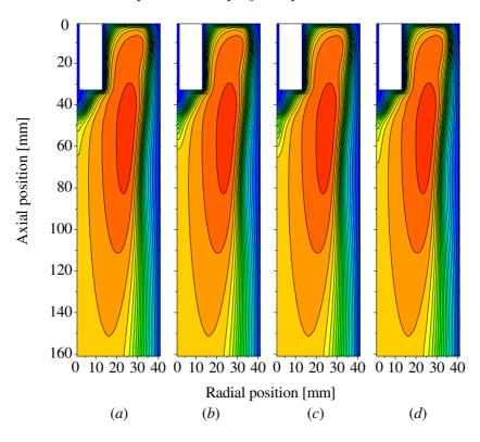
**Figure 17.** Temperature distribution of Ar thermal plasma with polymer solid powder injection. Thermodynamic and transport properties of Ar are used imaginarily for those of polymer-ablated vapours instead of their real polymer vapour properties. (a) PTFE; (b) PMMA; (c) PE; (d) POM.
