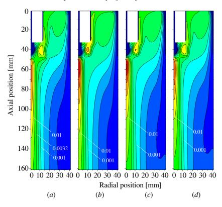
**Figure 11.** Mass fraction distribution of polymer-ablated vapours in Ar thermal plasmas at atmospheric pressure. The powder feed rate is 1 g min<sup>-1</sup>. (a) PTFE (b) PMMA (c) PE (d) POM injection cases.
