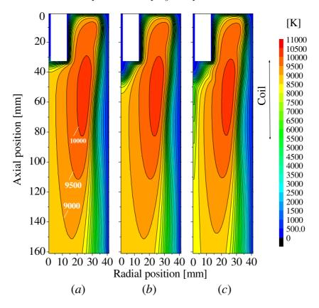
**Figure 8.** Temperature distribution of Ar thermal plasmas at atmospheric pressure with input power of 30 kW. (a) with Ar sheath gas; (b) with Ar sheath and centre carrier gases; (c) with Ar sheath and centre carrier gases, and PTFE powder injection at a feed rate of 1 g min<sup>-1</sup>.
