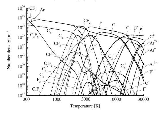
**Figure 4.** Equilibrium composition of 50%Ar-50% PTFE ablated vapour at atmospheric pressure.
