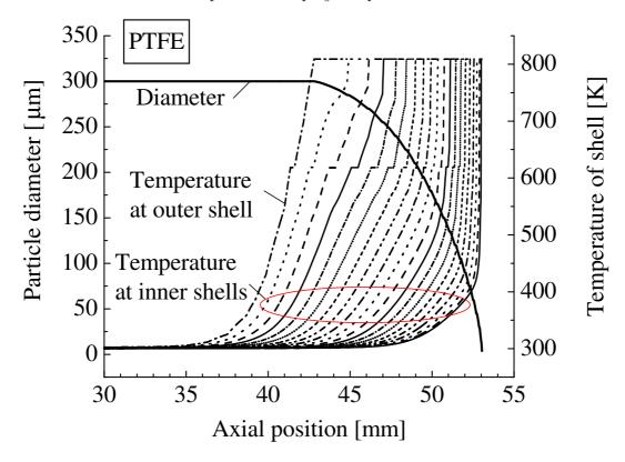
Figure 7. Temperature variation in each shell inside a test PTFE particle injected into Ar thermal plasmas.
