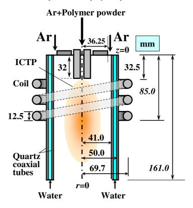
Figure 2. Plasma torch configuration and calculation space.
