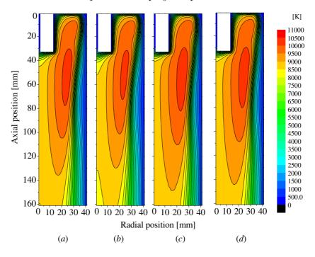
**Figure 18.** Temperature distribution of Ar thermal plasma with 0.1% premixed polymer-ablated vapour. No centre gas is fed. (a) PTFE (b) PMMA (c) PE (d) POM
