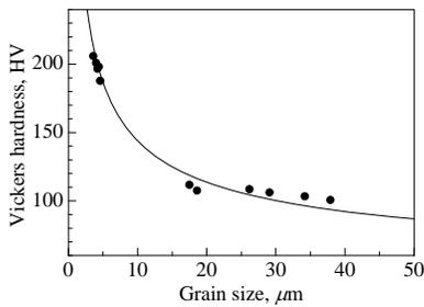
Fig. 3. Relation between grain size and Vickers hardness.
