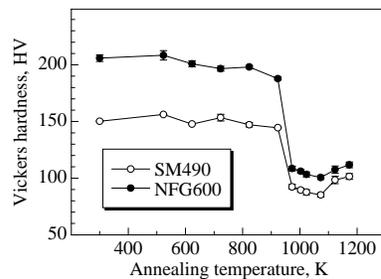
Fig. 2. Relation between annealing temperature and Vickers hardness.
