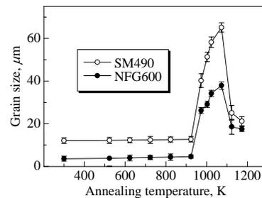
Fig. 1. Relation between annealing temperature and grain size
