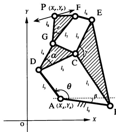
(b) 6-bar planar mechanism
