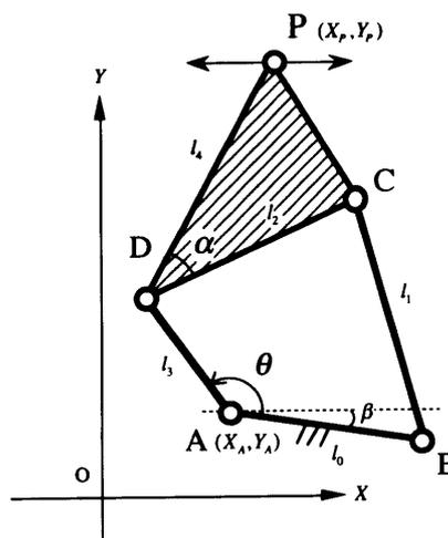
(a) 4-bar planar mechanism
