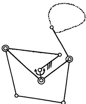
Fig. 13 Obtained 6-bar planar mechanism (Curve 2)
