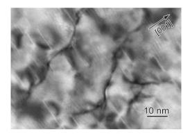
**Figure 1.** TEM image of disk-shaped  $\gamma''$  precipitates in a Cu-1.2%Ni-0.2%Be alloy aged at 450°C for 2 h after 40% cold-rolling. The zone axis is [110]<sub> $\alpha$ </sub>.
