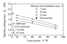
Fig.5 Influence of laser power on specific cutting force
