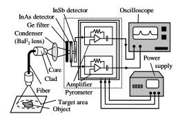
Fig.4 Schematic illustration of two-color pyrometer
