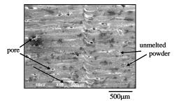
Fig.2 SEM image of the consolidated surface
