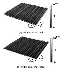
Fig.8 Comparison of the processed surface
