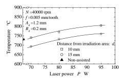
Fig.7 Influence of laser power on tool temperature
