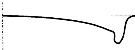
Fig. 15 Deformed shell when buckling
