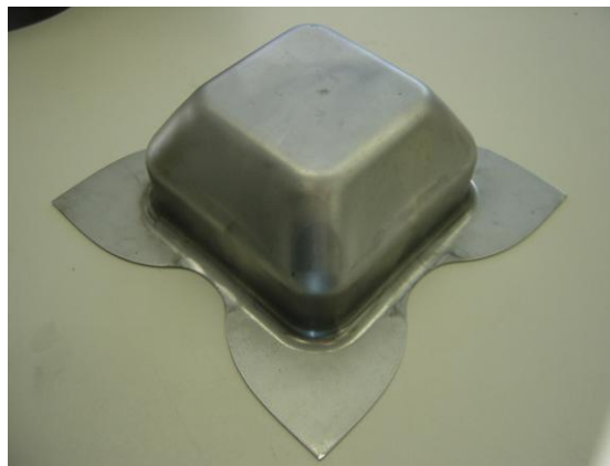
Fig.15 The square cup deep drawing in the experiment (Initial BHF=20 kN)
