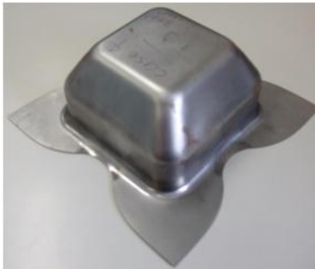
Fig.2(a) Molding in experiment
