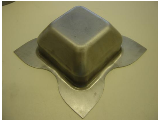
Fig.18 The square cup deep drawing in the experiment (Initial BHF=100 kN)
