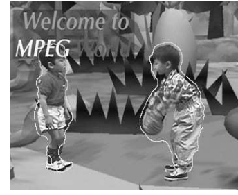
Fig. 2. Extraction from the Frame Difference using the LoG Filter.
