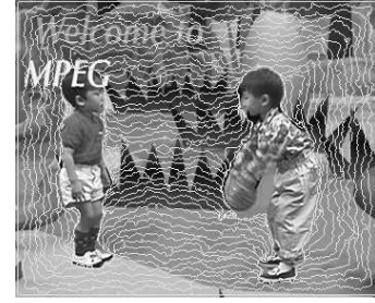
Fig. 3. Locus of Contour Obtained by the Speed Function using the Frame Difference.
