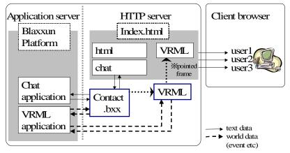
Fig. 1. System framework with the Blaxxun platform
