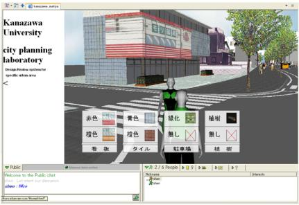
Fig. 11. The tool with a panel for switching and coordinating design alternatives for review
