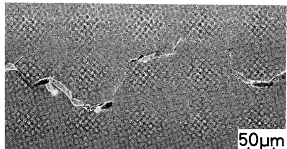
(c) K=31.0\text{MPa}\sqrt{\text{m}} d=172\mu\text{m}
