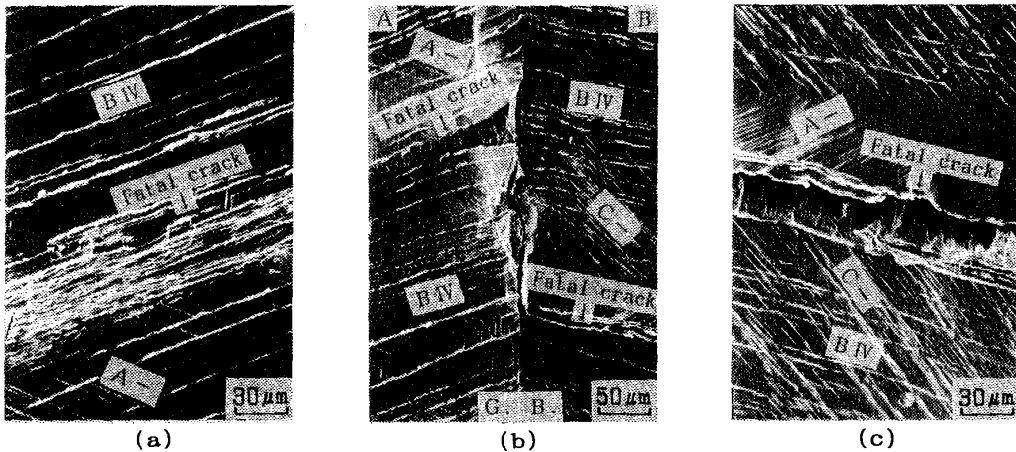
Fig.5 Fatal crack in bicrystal B1 at (a) component crystal A, (b) grain boundaly and (c) component crystal B. ( N=1.6 \times 10^5 )
