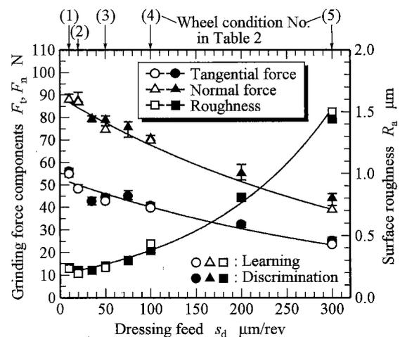
Fig. 5 Variations of grinding force components and surface roughness with dressing conditions
