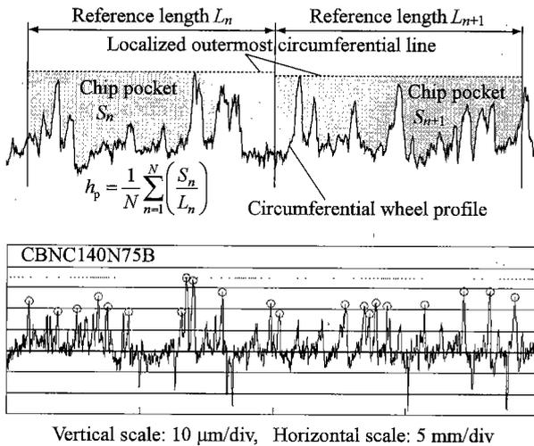
Fig. 8 Definition of average depth of chip pocket  $h_p$  and typical wheel profile
