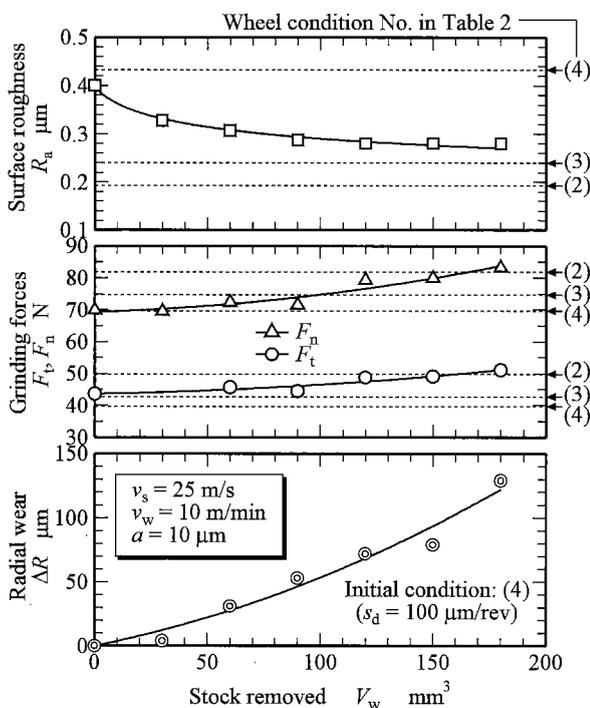
Fig. 6 Variations of grinding force components, surface roughness and radial wheel wear with accumulated stock removed
