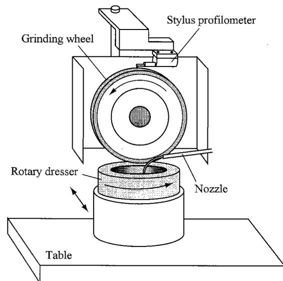
Fig. 7 Rotary dresser and stylus profilometer
