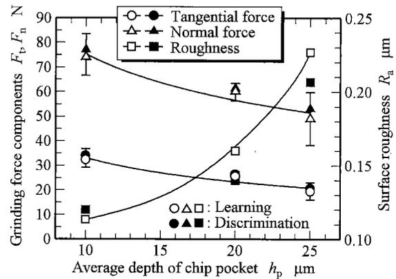
Fig. 10 Variations of grinding force components and surface roughness with depth of chip pocket for resinoid-bonded CBN wheel
