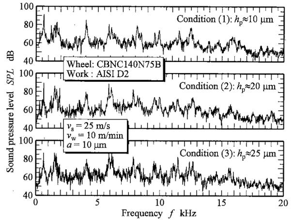
Fig. 2 Typical frequency spectra of the grinding sounds for three grinding wheel conditions
