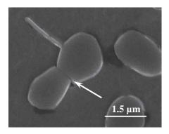
(a) Crack in cementite particle
