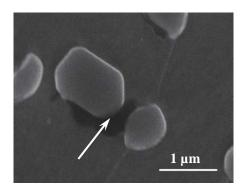
(b) Crack separation between cementite particle and matrix Figure.16 Crack in particle and at the boundary
