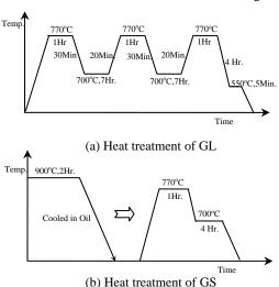
Figure.4 Heat treatment process
