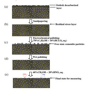
Figure.6 Surface treatment procedure
