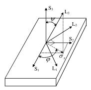
Figure.1 Coordinates of X-ray stress measurement
