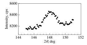
Figure.8 Intensity of the 250 cementite peak ( $\psi$ =0)
