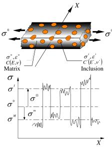
Figure.2 Stress in two-phase composite material
