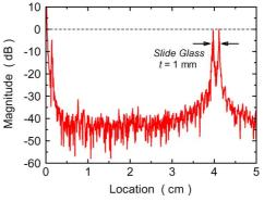
Fig. 5. Measured reflection profile for an 1-mm-thick slide glass located at 4 cm.
