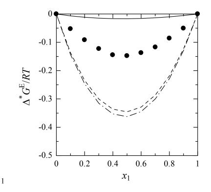
Figure 4. Excess Gibbs energy of activation for the system phenylmethanol (1) + 2-butanone (2) at T =3 303.15 K: •,  $\Delta^* G^{\text{E}}_{\text{exp}}/RT$ ; --,  $\Delta^* G^{\text{EC}}_{\text{cal}}/RT$ ; --,  $\Delta^* G^{\text{ER}}_{\text{cal}}/RT$ ; --,  $\Delta^* G^{\text{E}}_{\text{cal}}/RT$ .
