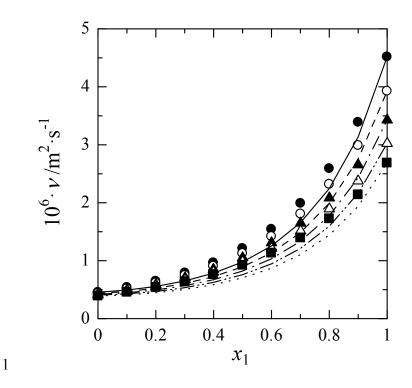
Figure 3. Kinematic viscosities for the system phenylmethanol (1) + 2-butanone (2): ●, v<sub>exp</sub> at 303.15
