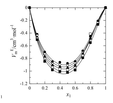
Figure 1. Excess molar volumes for the system phenylmethanol (1) + 2-butanone (2): ●, 303.15 K; ○,
