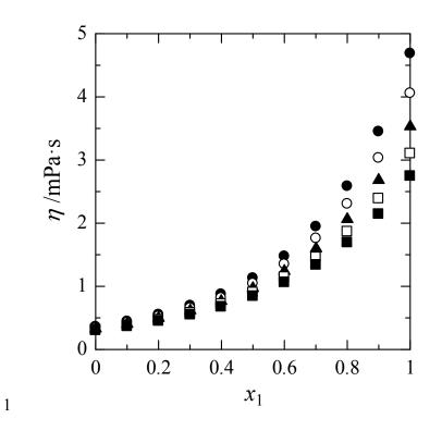
Figure 2. Experimental viscosities for the system phenylmethanol (1) + 2-butanone (2): ●, 303.15 K;
