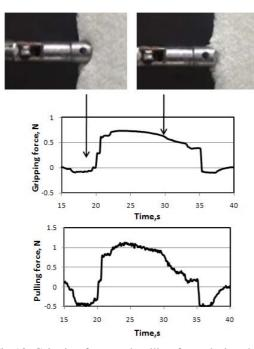
Fig.18. Gripping force and pulling force during the grasping and pulling soft material
