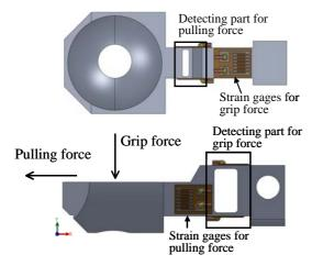
Fig.3. Detail structure of the force detecting clip
