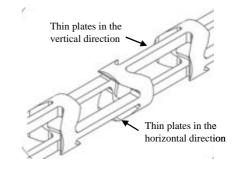
Fig.10. Flexion structure of the inner pipe
