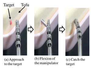
Fig.17. Operation test to catch a target on the soft material surface
