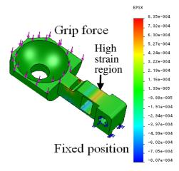
Fig.4. Strain analysis on the detection clin
