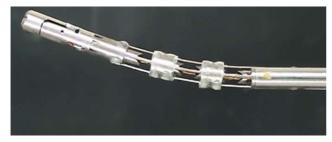
Fig.13. Flexion of the assembled micro manipulator by pulling the wire through the outer pipe
