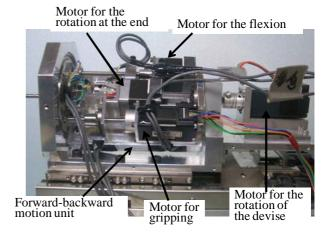
Fig.15 Slave manipulator driving devise
