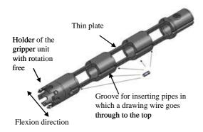
Fig.8. Structure of the flexible outer pipe
