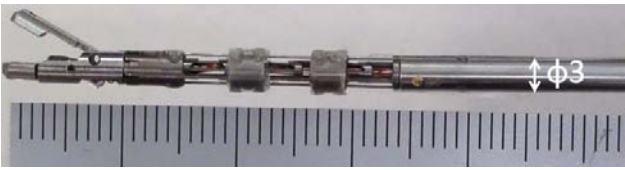
Fig.12 Assembled gripper and micro manipulator
