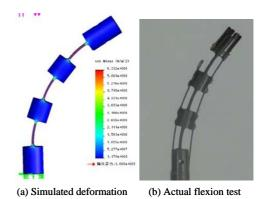
Fig.9. Deformation analysis and actual deformation of the outer pipe
