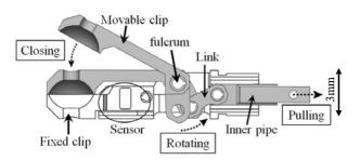
Fig.2. Setup of the gripper
