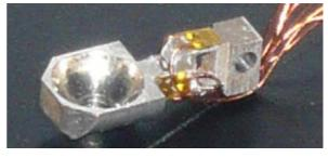
Fig.5. Manufactured clip and fit strain gages
