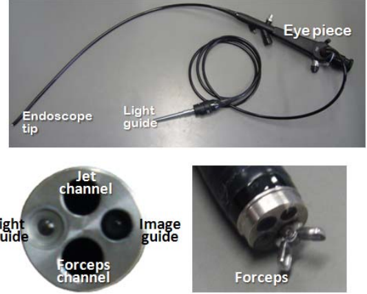
Fig. 2 Photographs of the newly designed endoscope
