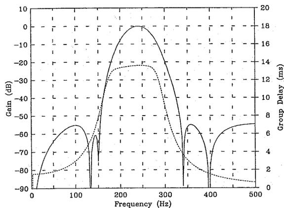
Figure 12: Characteristics of the third IF filter
