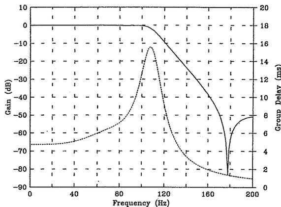
Figure 8: Characteristics of the 100-Hz low-pass filter for ELF
