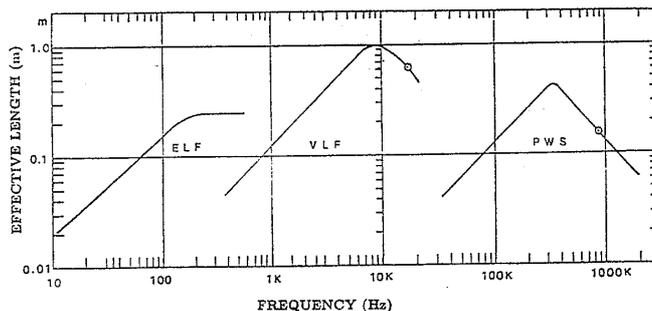
Figure 4: Frequency dependence of the effective length of the loop antennas and search coils [Kimura et al., 1990]
