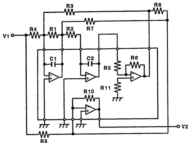
Figure 7: Biquad filter IC
