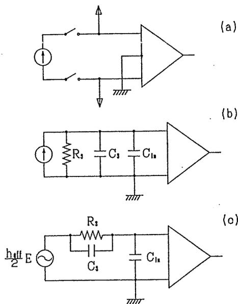
Figure 9: Basic equivalent circuits of VIP
