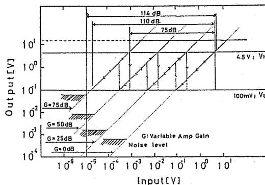
Figure 6: Gain characteristics of the WIDA IC
