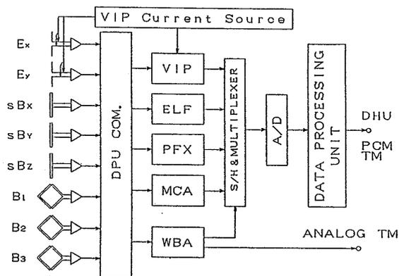
Figure 1: Block diagram of the VLF instrument
