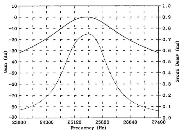
Figure 11: Characteristics of the first IF filter
