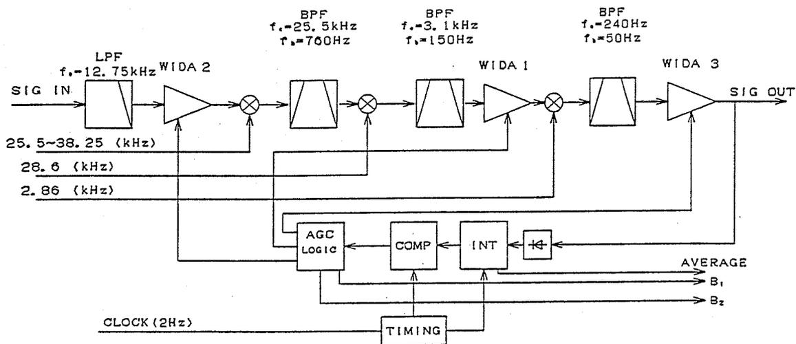
Figure 10: Block diagram of the PFX
