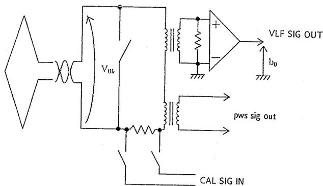
Figure 3: Block diagram of the loop antennas and pre-amplifier
