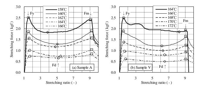
Fig.5 Stress -strain curve of (a) sample A and (b) sample V at several stretching temperatures
