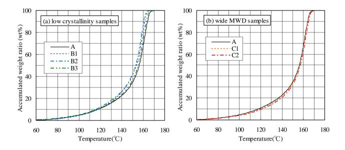
Fig.10 Accumulated weight ratio of the melting parts on DSC (wt%)
