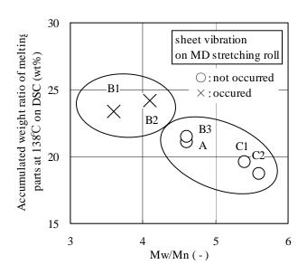
Fig.11 Sheet Vibration on the MD stretching roll
