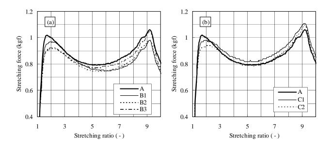
Fig.8 Strain-Stress curve of (a)low crystallinity samples and (b)wide MWD samples
