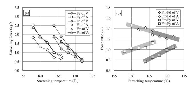
Fig.7 (a) Stretching force and (b) stretching force ratio of sample A and V
