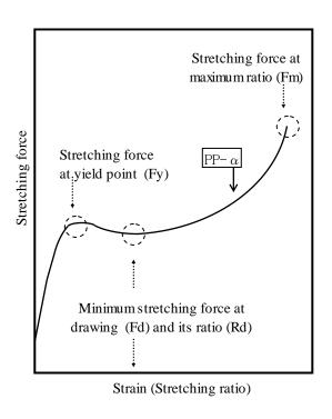
Fig.4 The definition of stretching parameters of Fy, Fd, Rd and Fm
