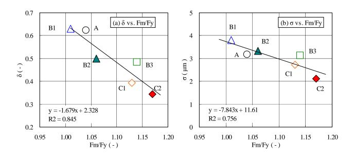
Fig.12 Relationship between Fm/Fy and film thickness uniformity parameter (a) $\delta$ , (b) $\sigma$
