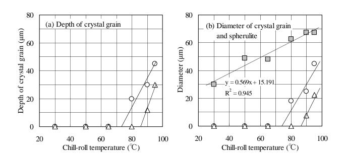
Fig.11 Crystal structure of PP sheets with different chill-roll temperatures
