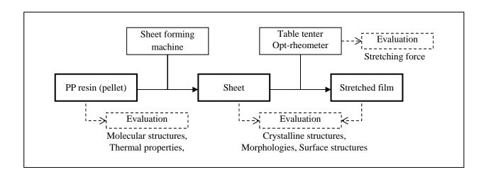
Fig. 2 Diagram production and evaluation methods of each sample
