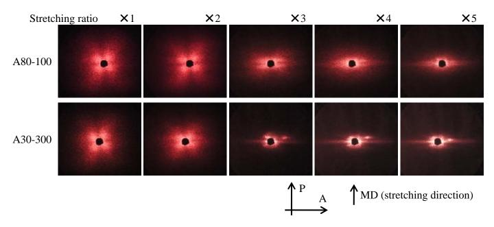
Fig.16 Light scattering patterns stretched by opt-rheometer obtained from PP sheets with different chill-roll temperatures
