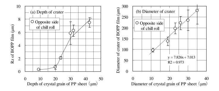
Fig.8 The relationship between crystal structure of PP sheets and crater structure of BOPP films
