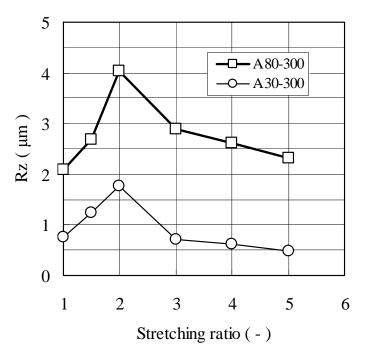
Fig.15 Rz of BOPP films stretched by opt-rheometer obtained from PP sheets with different chill-roll temperatures
