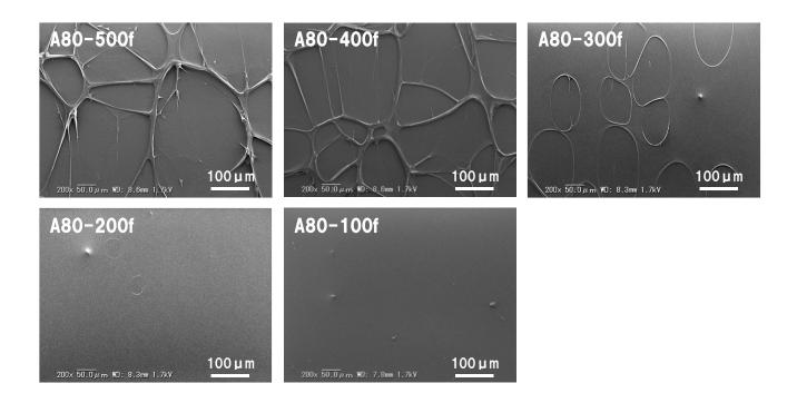
Fig.6 SEM images of BOPP films surface of opposite side of chill-roll, obtained from PP sheets with different thicknesses
