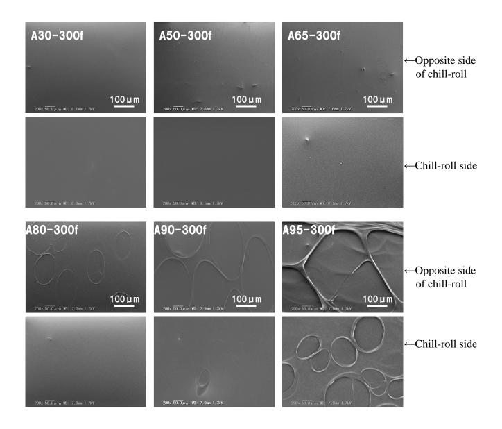
Fig.13 SEM images of BOPP films surface obtained from PP sheets with different chill-roll temperatures
