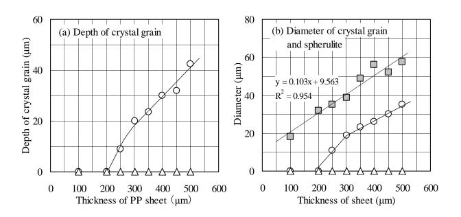
Fig. 4 Crystal structure of PP sheets with different thicknesses
