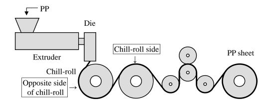
Fig. 1 Schematic diagram of PP sheet forming machine
