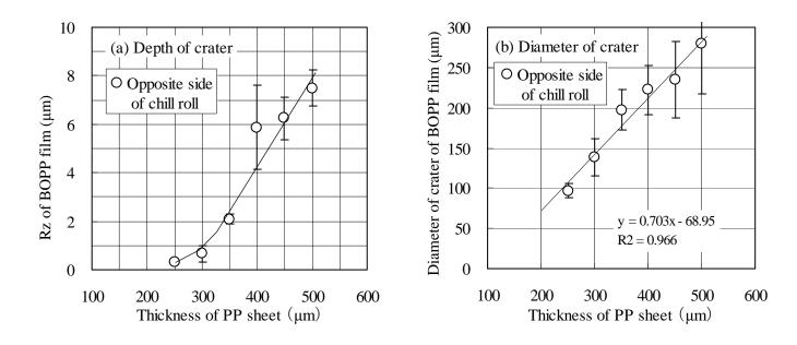
Fig.7 The relationship between PP sheet thickness and crater shape
