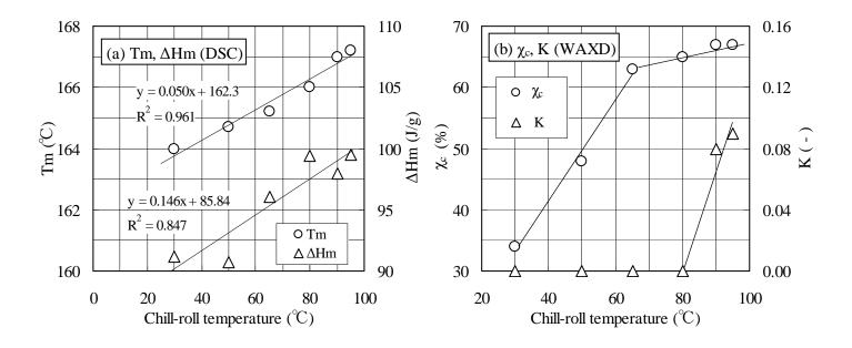
Fig.12 Properties of PP sheets with different chill-roll temperatures measured by (a) DSC and (b) WAXD
