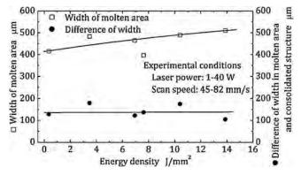
Fig. 8. Variation of molten width and shrunk distance with energy density.
