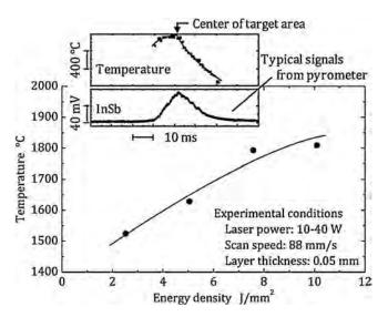
Fig. 5. Variation of temperature with energy density.
