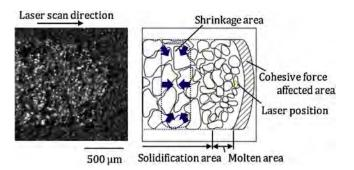
Fig. 7. Consolidation aspect of metal powder.
