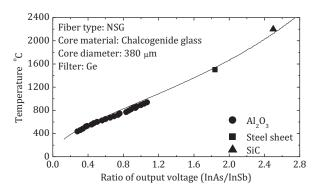
Fig. 2. Calibration curve obtained.
