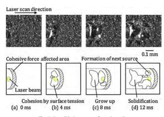
Fig. 4. Consolidation aspect of metal powder.
