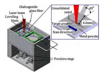
Fig. 3. Experimental setup for temperature measurement.
