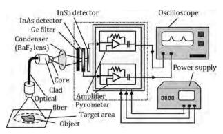
Fig. 1. Fundamental structure of two-color pyrometer.
