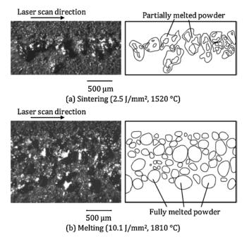
Fig. 6. Comparison of the influence of energy density on consolidation.
