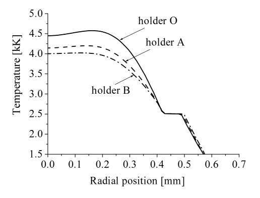
Figure 6. Radial distributions of the Hf cathode surface temperature for different cathode holder shapes.
