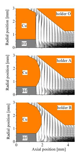
Figure 7. Gas flow fields with different cathode holder shapes.
