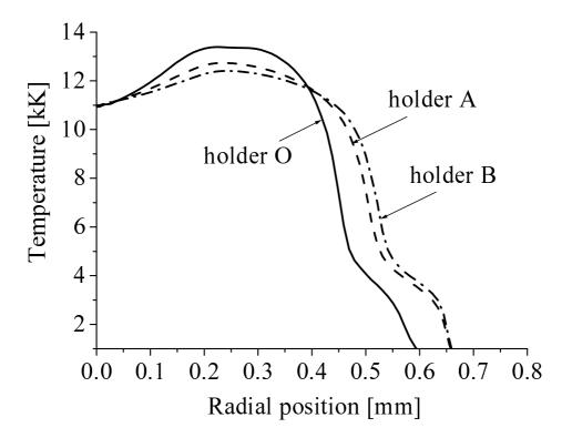
**Figure 4.** Radial distributions of the arc plasma temperature near the cathode surface for different cathode holder shapes.
