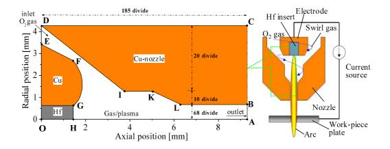
Figure 1. Schematic diagram of plasma cutting torch
