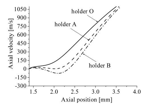
Figure 8. Axial distributions of velocity along the center axis for different cathode holder shapes.
