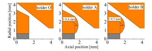
Figure 2. The shape of cathode holder.
