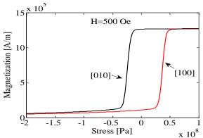
Fig. 3. Magnetization curves under uniaxial mechanical stress.
