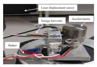
Fig. 9. Measurement setup
