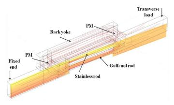
Fig. 2. The 3-D model of the Galfenol unimorph vibration energy harvester.
