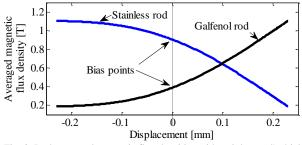
Fig. 8. Rod-averaged magnetic flux densities with stainless rod's thickness of  $0.5\,\mathrm{mm}$ .
