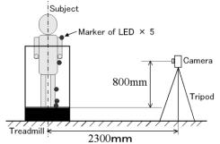
Fig.4. Walking measurement system
