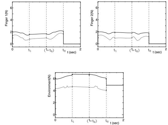
Figure 7: Simulation Result of Pivoting (norm of force)
