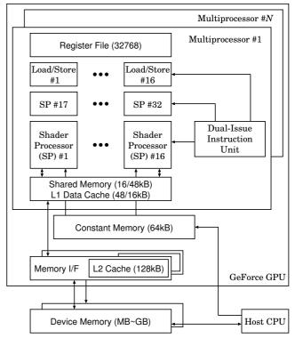
Figure 2: Computation model for Fermi architecture
