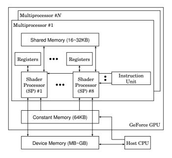
Figure 1: Computation model for Tesla architecture
