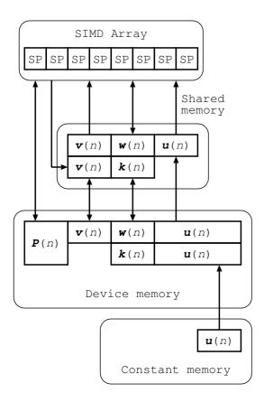
Figure 3: Memory assignments for small filter
