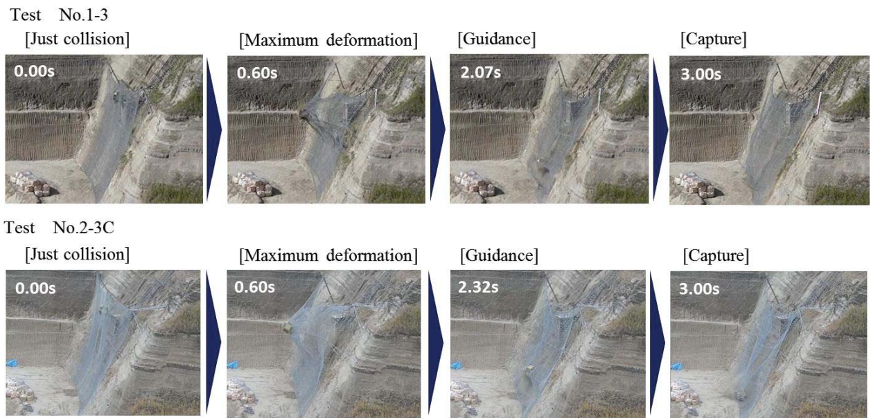
Fig.6: Test No.1-3 and No.2-3C according to high-speed photography
