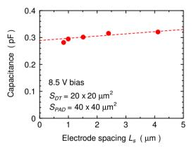
(b) Relation between electrode spacing and capacitance.
