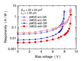
Fig. 4 Responsivity against bias voltage of CMOS-APDs.
