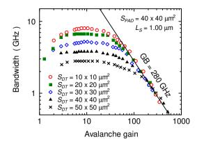
**Fig. 10** Relation between avalanche gain and bandwidth of the CMOS-APDs for different detection area  $S_{DT}$ .
