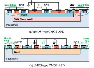
Fig. 2 Cross-sectional structure of fabricated CMOS-APDs.
