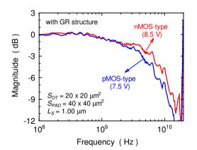
Fig.7 Comparison of frequency response of nMOS-type and pMOS-type CMOS-APD with GR.
