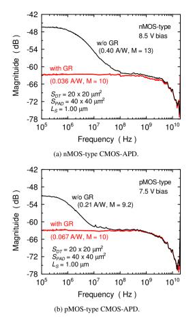
Fig. 6 Frequency response of CMOS-APDs with and without GR.
