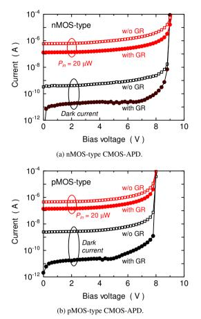
**Fig.3** *I–V* characteristics of CMOS-APDs with and without GR. The electrode spacing  $L_S = 1.0 \,\mu\text{m}$  and the detection area  $S_{\text{DT}} = 20 \times 20 \,\mu\text{m}^2$ .
