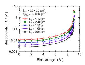
**Fig. 5** Responsivity of nMOS-type CMOS-APDs with the GR for different electrode spacing  $L_S$ .
