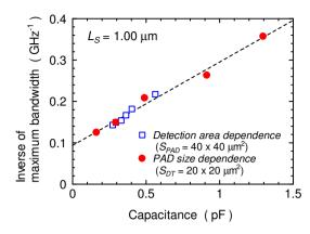
Fig. 13 Relation between the device capacitance and the inverse of the maximum bandwidth of the CMOS-APDs.
