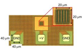
Fig. 1 Photograph of fabricate CMOS-APD.
