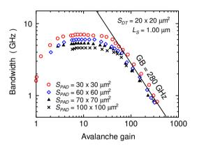
Fig. 11 Relation between avalanche gain and bandwidth of the CMOS-APDs for different PAD size  $S_{PAD}$ .
