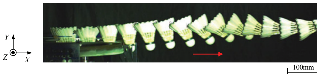
Fig. 11 After launch ( \gamma=0^\circ ), the flight behavior of the shuttlecock captured using a high-speed video is shown. This stroboscopic image is captured at every 2ms/frame. Initial velocity of the shuttlecock is 29.4 m/s.
